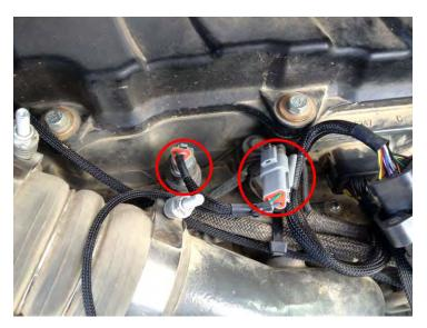
**6)** Route the power and ground wires over the top of the engine to the alternator, located on the opposite side. Connect the red wire to +12 volts and the black wire to ground.
