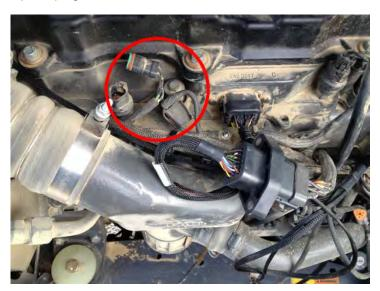
**5)** Plug the male connector from the Ag Diesel Solutions harness into the stock MAP Sensor. Plug the female connector from the Ag Diesel Solutions harness to the stock connector that was removed from the MAP Sensor.
