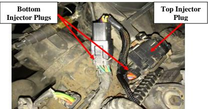
3) Disconnect the stock female Injector Harness plug located on the Top. Connect the female plug from the Performance Module Harness into the male Injector Harness Plug. Connect the stock female Injector plug into the corresponding male Harness plug on the new Harness. \*Note: Use the Injector Connector on the Performance Module Harness marked "Top". The connectors on the module harness are Grey that connect to the Top plug.
