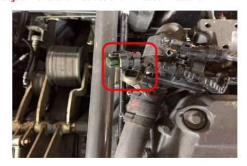
**6)** Plug the female connector from the module harness into the male exhaust pressure sensor plug. Plug male connector from module harness into the female exhaust pressure sensor plug.
