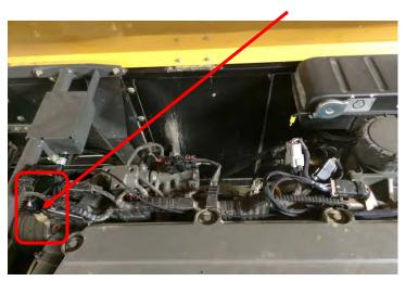
5) Disconnect the stock Exhaust Pressure Sensor.
