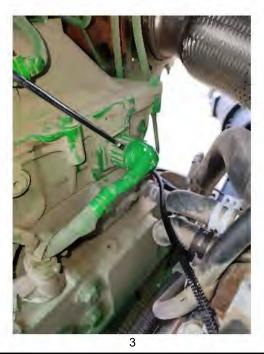
2) Plug male module connector into factory female connector in cylinder head. Plug female module connector into male factory harness connector.
