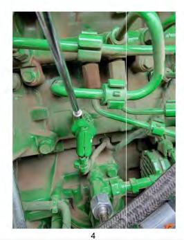
**4)** Plug the module male connector into the MAP sensor. Plug module female connector into factory harness male connector.
