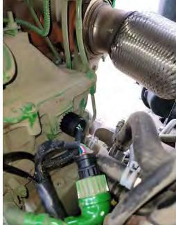
**3)** Locate MAP sensor located directly under fuel rail, on left side of engine.
