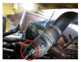
4) Locate injector connectors and unplug.
