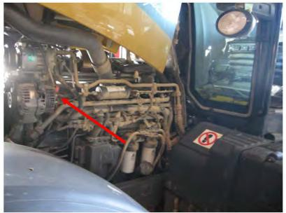
8) Mount the module with the connector on the bottom side, as to reduce the chance of moisture from getting into the module harness. Keep away from excessive heat and moving parts. Note: Zip tie onto the factory computer wire harness works well. Mounting the module as shown will help prevent moisture from collecting into the module connector.
