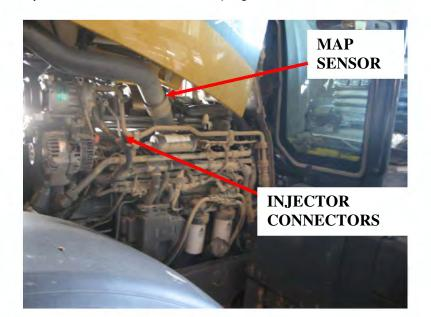
**3)** Plug MAP sensor connector from the Ag Diesel Solutions module into the MAP sensor and plug the MAP harness from engine into module.
