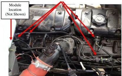
**5)** Connect the red wire with ring terminal to a +12V constant source. Connect the black wire with ring terminal to a good chassis ground.
