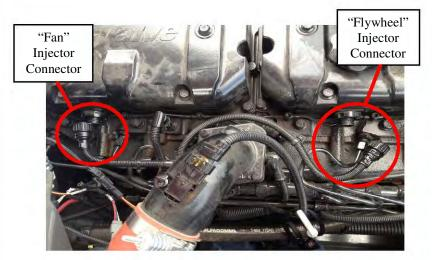
**3)** Facing the side of the engine, route the module harness as shown in the pictures below. The module connector will be located to the left of the injector connector labeled "fan" in Step 1.
