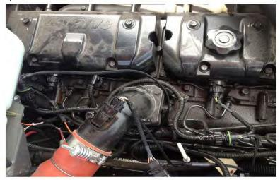
**4)** On the module harness, the male injector connector located closest to the module will plug into the "fan" injector connector on the engine head. The male injector connector located farthest from the module will plug into the "Flywheel" connector on the engine head. The male connectors plug into the stock injector plugs removed in Step 2.
