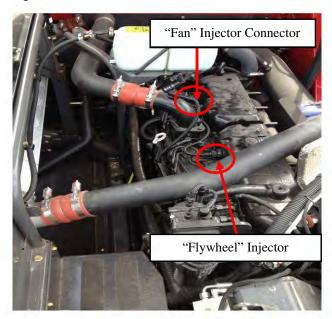
**2)** Rotate the outer collar of the injector connectors counterclockwise to disconnect both fan and flywheel side connectors.
