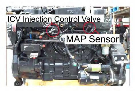
2) Connect the male injection control valve connector from the module into the stock female connector.
