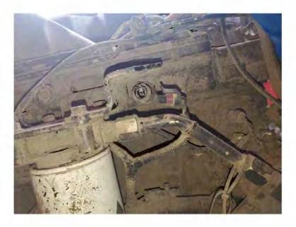
**5**) Connect the Female MAP sensor connector from the Ag Diesel Solutions harness into the stock male MAP sensor connector.
