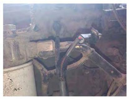
**6)** Connect the red wire with a ring terminal to a constant 12 volt source. Connect the black wire with a ring terminal to a good engine ground. Wiring can be routed over the engine to the Alternator. Note: For RV's, power and ground needs to be connected to the engine, not the house battery system.
