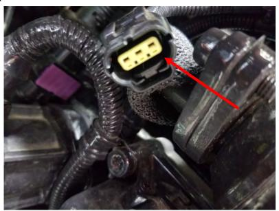
**4)** Plug Female Fuel Pressure Connector from module into fuel pressure sensor.
