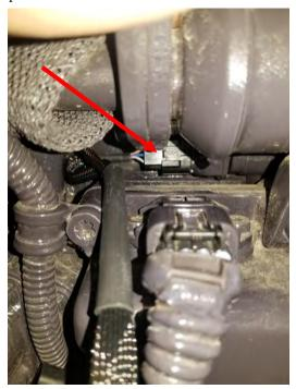
5) Connect the Stock Cummins connector to the Male Fuel Pressure Connector on the module harness.
