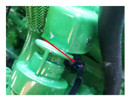
5) Connect the Stock Cummins connector to the Male Fuel Pressure Connector on the module harness.
