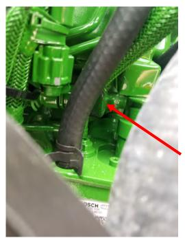
3) Press on release tab and pull away from fuel rail to unplug the fuel pressure sensor connector.
