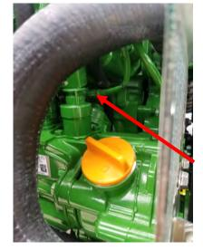
2) Locate fuel pressure sensor as shown below. It can be found at the end of the fuel rail closest to the fan.
