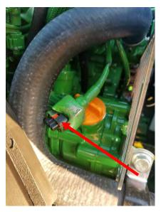
**4)** Plug Female Fuel Pressure Connector from module into fuel pressure sensor.
