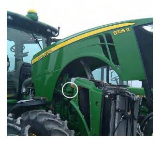
2) Locate the injector connector.
