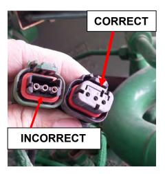
8) Plug the stock MAP sensor connector into the male MAP sensor connector on the Ag Diesel Solutions Module.
