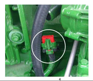
**4)** Plug the stock male connector into the Ag Diesel Solutions harness.
