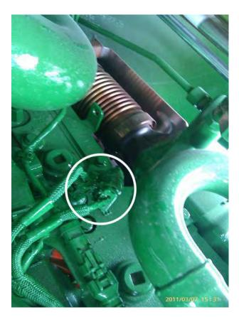
Note: There are two similar connectors, ensure the module is connected to the MAP sensor circled below.
