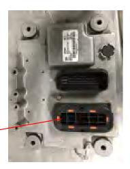
5) Disconnect both ECM connectors by rotating the locking lever to release and Move out of way.
