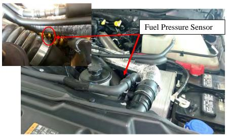
2) Unplug the fuel pressure sensor. It is located at the end of the common fuel rail. The common fuel rail runs alongside the valve cover.
