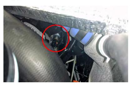
3) Plug male connector from module into fuel pressure sensor. Plug the stock connector to the female connector from the module.
