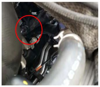
**4)** Below are photo examples representing how the factory fuel rail sensor plug should be connected to our 3-Pin female connector on the ADS module harness.
