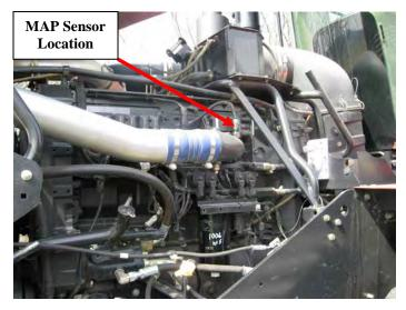
Locate MAP sensor on left side of engine in the air intake manifold
