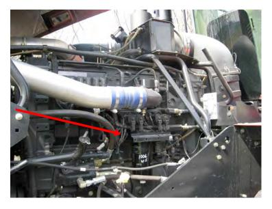
Locate Fuel Quantity Valve sensor as shown in Picture
