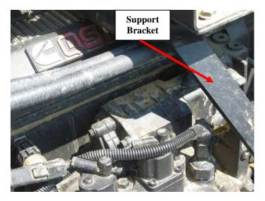
**10)** Mount the module box in a safe location using the zip ties to secure the wires and module away from any extreme heat and moving parts. A good location to mount the module is on the given support bracket.
