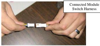
**8**) Remove the bypass plug from the Ag Diesel Solutions harness, and plug the harness into the module.
