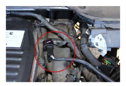
5) Locate the MAP Sensor. It is located on the intake on the driver's side of engine under the fuel rail.
