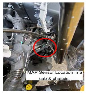
**6)** Disconnect the stock MAP Sensor. Plug the male connector from the module into the stock MAP Sensor. Plug the female connector from the module into the stock wiring harness.
