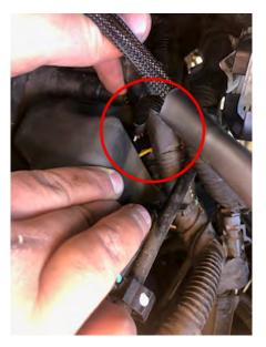
**4)** Connect the stock fuel pressure connector to the female connector from the module.
