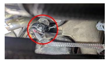
**5)** Following, connect the stock 4-pin male connector to the female 4-pin connector from the module harness. Insure that all connections snap into place as well as re-locking the grey connector tabs on both ends of the harness.
