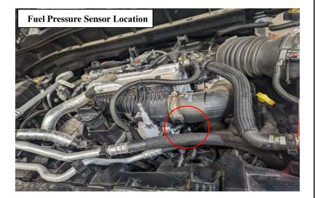
**2)** Locate the fuel rail pressure sensor on the end of the fuel rail towards the front of the engine.
