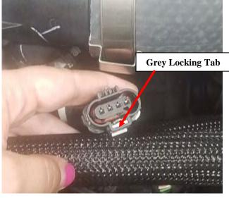
**4)** Insert the 4-pin male connector from module harness into fuel pressure sensor.
