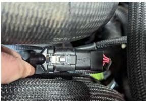
**6)** Remove the bypass plug from the Ag Diesel Solutions harness, and plug the harness into the module. Note: Keep the bypass plug for potential troubleshooting.
