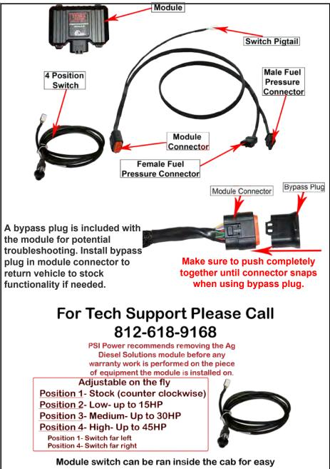
Module switch can be ran inside the cab for easy performance adjustment. Module switch can be secured in engine bay if desired. Module will default to HIGH setting if switch is not connected
