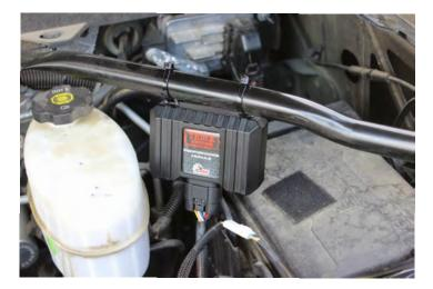
**8)** Connect module switch harness. Based on preference, the module switch can be secured in the engine compartment near the module or it can be routed into the cab. If mounting in the cab, route the switch through the firewall and connect to the module harness.
