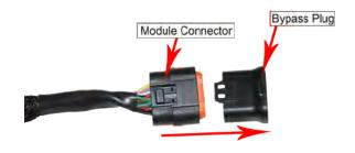
7) Re-install all components removed for the installation process. Mount the module box in a safe location using the zip ties to secure the wires and module away from any extreme heat and moving parts. Note: Zip tie the module to the factory wire harness. Mounting the module with the connector down will help prevent moisture from collecting into the module connector.
