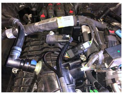
7) Remove the bypass plug from the Ag Diesel Solutions harness, and plug the harness into the module.
