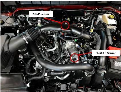
**2)** Remove the 10mm bolt and loosen bracket to gain access to the MAP sensor.
