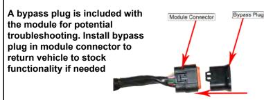
Make sure to push completely together until connector snaps when using bypass plug.
