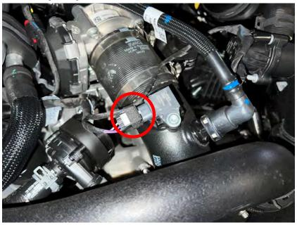
**6)** Utilize the portion of the Ag Diesel Solutions harness labeled T-MAP. Connect the male connector to the T-MAP Sensor. Then connect the female connector to the stock male T-MAP Sensor connector.
