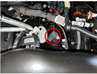
**4)** Utilize the portion of the Ag Diesel Solutions harness labeled MAP. Connect the male connector to the MAP Sensor. Then connect the female connector to the stock male MAP Sensor connector.
