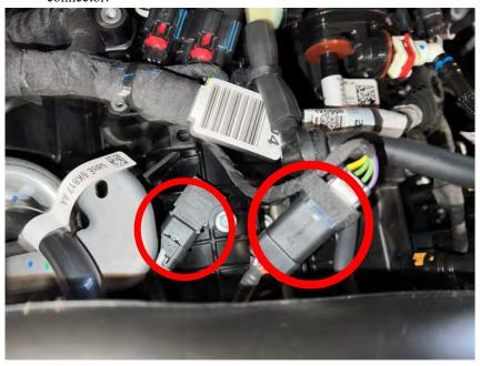
**5)** Disconnect stock T-MAP sensor connector by pulling back on locking tab and squeezing the connector release tab.
