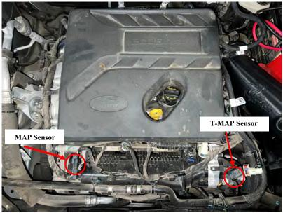
2) Disconnect stock MAP sensor connector by pulling back on locking tab and squeezing the connector release tab.
