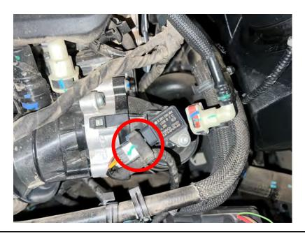
**5)** Utilize the portion of the Ag Diesel Solutions harness labeled T-MAP. Connect the male connector to the T-MAP Sensor. Then connect the female connector to the stock male T-MAP Sensor connector.
