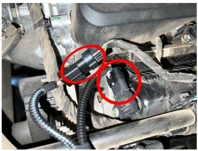
**4)** Disconnect stock T-MAP sensor connector by pulling back on locking tab and squeezing the connector release tab.
