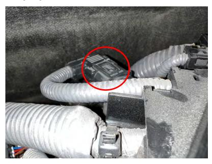
**3)** Connect the ADS female MAP connector to the factory MAP sensor. Connect the ADS male MAP connector to the factory female MAP sensor connector.
