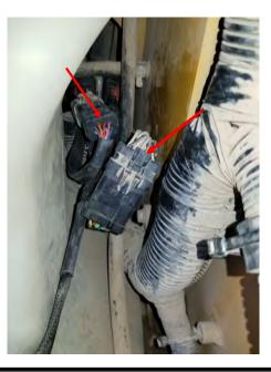
**6)** Route power and ground leads along factory wiring loom to the battery. Connect red wire with ring terminal to positive battery post. Connect the Black wire with ring terminal to negative battery post.
