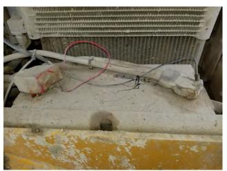
**7)** Mount the module with the connector on the bottom side, as to reduce the chance of moisture from getting into the module harness. Keep away from excessive heat and moving parts.
