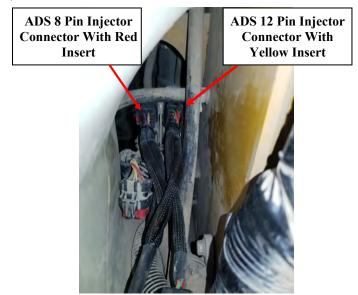
**5)** Plug the male ADS injector connectors into the factory female injector connectors. Again matching pin count and insert color.
