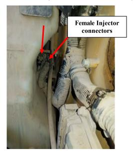
**3)** Unplug the two factory injector connectors shown by pulling back on the lock tab and depressing the release just forward of the lock. One connector will be a 12 pin with yellow insert, the other 8 pin with a red insert.
